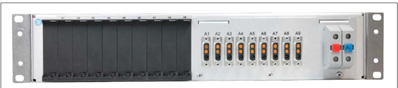
fig. 3: front view PDB-N-CP09A-FF-Ax terminals on the front with high current SUB-D connectors
